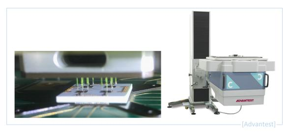
Transceiver front-ends for millimeter-wave wireless communications, such as driven by 5G and 6G systems, are increasingly integrated together with antenna arrays within compact module form factors. The production test and calibration of such modules requires new over-the-air (OTA) measurement concepts. This project shall investigate new OTA concepts, addressing electromagnetic and antenna aspects as well as strategies and requirements for test and calibration of large arrays.
